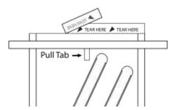
2. Tear off the top of both bags where indicated. Put aside the empty bag. Pull tabs to open the sponge bag. If needed, add a collection solution to hydrate the dry sponge device.
