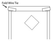
12. Roll down the top of both bags several times and fold down the wire ties to close. Send both sample bags to laboratory for analysis.
