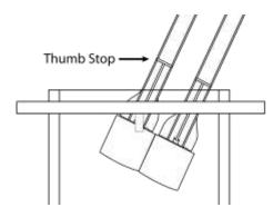
3. Keeping hands outside the bag, guide the handles out the top of the bag. Grasp the handles above the thumb stop and remove the device.
