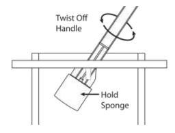
11. Transfer the 2nd device into the empty sample bag. Do not insert past thumb stop. With hands outside the bag, twist off the handle in a counter-clockwise direction.
