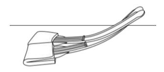
5. Press down firmly and flex the handle to ensure the entire sponge paddle makes full contact with the sample surface.
