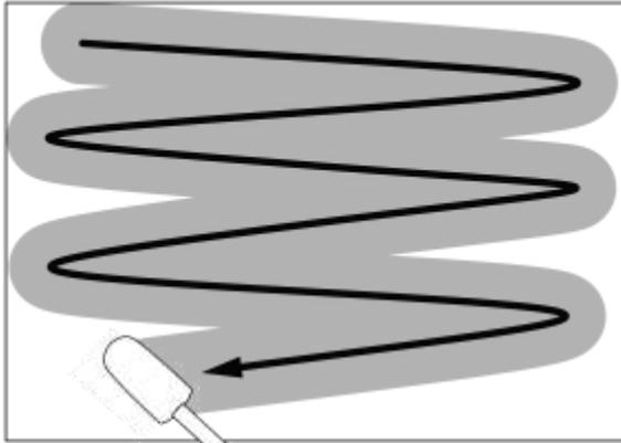
4. Vigorously scrub back and forth across the surface, while rotating the swab to ensure entire swab tip makes contact with the surface.
