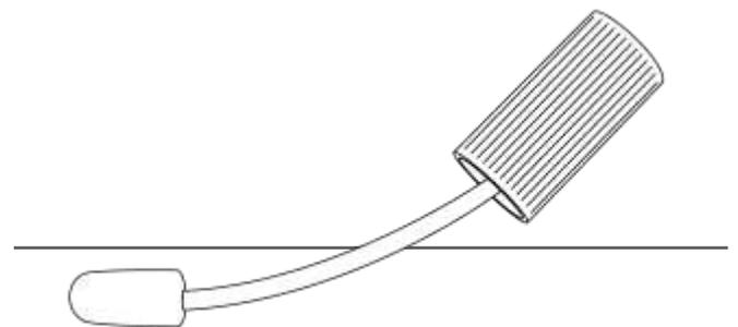
3. Press down firmly against surface to ensure the swab tip makes full contact with the sample surface.
