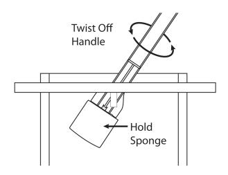
7. Return sampling device to the bag. Do not insert past the thumb stop. Hold sponge from the outside of the bag and twist off the handle by turning counter-clockwise.
