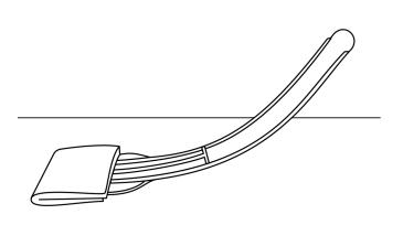
4. Press down firmly and flex the handle to ensure the entire sponge head makes full contact with the sample surface.
