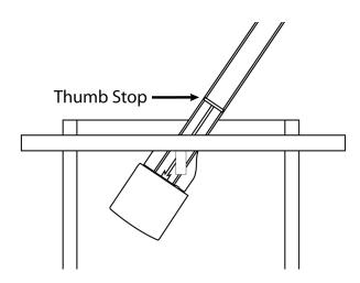
3. Keeping hands outside the bag, guide the handle out the top of the bag. Grasp the handle above the thumb stop and remove the device.
