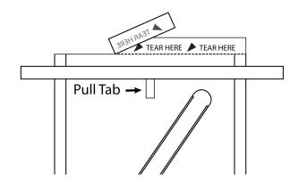
2. Tear off the top of the bag where indicated. Pull tabs to open bag. If needed, add a collection solution to hydrate the dry sponge device.
