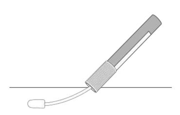
3. Press down firmly against surface to ensure the swab tip makes full contact with the sample surface.
