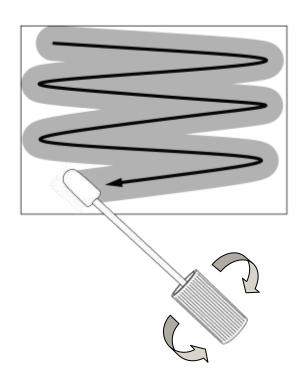
4. Vigorously scrub back and forth across the surface, while rotating the swab to ensure entire swab tip makes contact with the surface.
